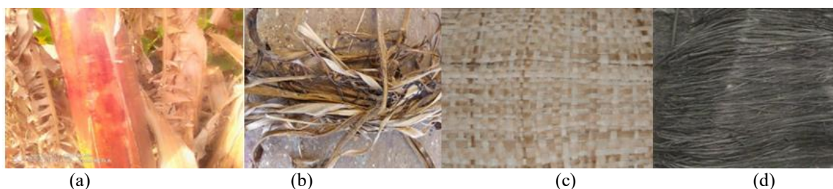
Plate 1: (a) Banana stem, (b) Strips from banana stem, (c) Extracted banana fibre (d) Banana fibre in mat form
